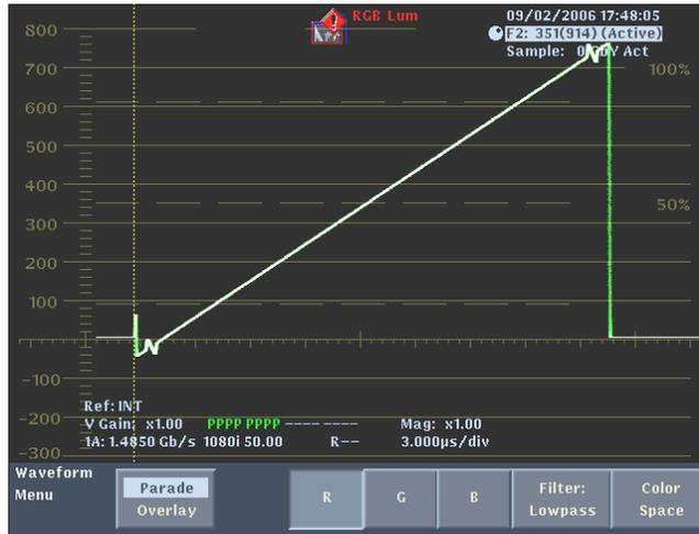
Figure 8 - A waveform showing levels below 0mV and above 700mV with a small notch (detail) in these sections.
